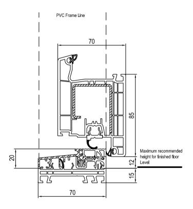
Note: 15 mm build up profile can be removed if not required. i.e. Polished Floor. 35 mm build up profile is also available.
